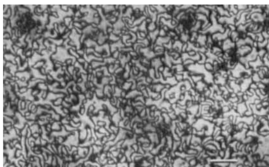
Figure 5. Photomicrograph taken of sample 4a between crossed polarizers at 25°C. Sample was annealed at approximately 230°C for several hours prior to cooling to 25°C. Bar shown in lower right corner is 40 \mu\text{m} long.
